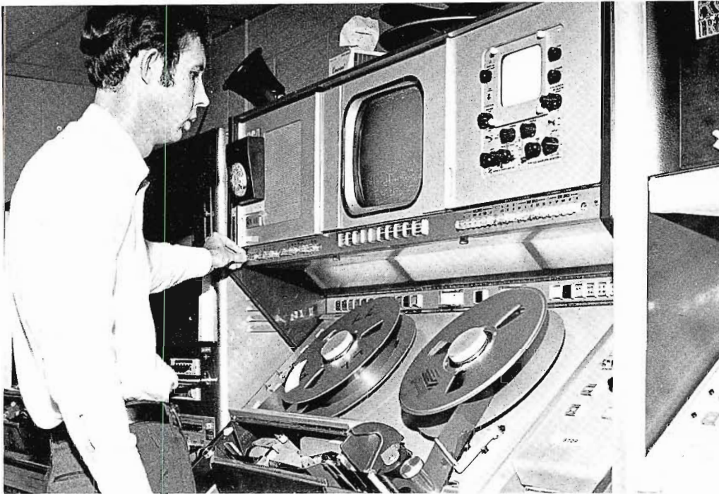
Addition of TCR-100 permits WFMY-TV to use TR-70 and other tape machines for production.
