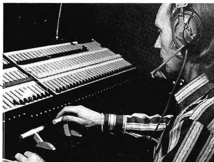
Time-saving remote dimmer lighting console features a 5-scene pre-set capability.
