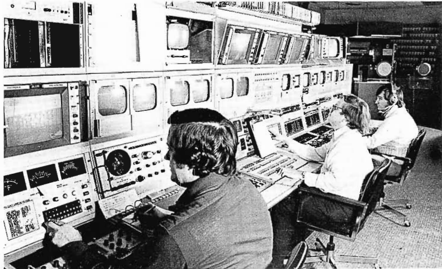
Compact control console line-up includes transmitter remote controls; switching and machine controls; and TK-44 CCU's.
